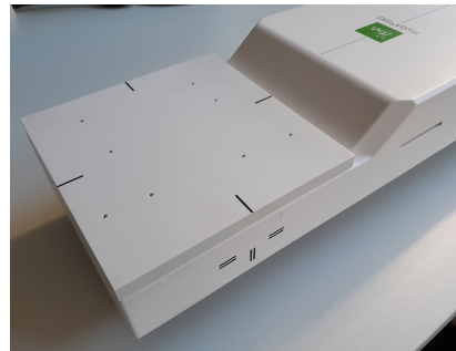
Fig. 3: myQA SRS array with the fiducial plate added on top of it
