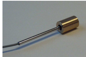
ii. A PFD 3 G -pSi diodes inside a brass build-up cap
