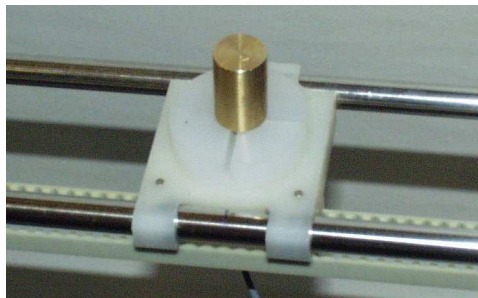
A brass build-up cap on a RFA holder
