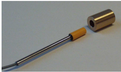
i. A PFD 3 G -pSi diodes and a brass build-up cap
