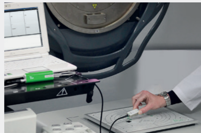
1) Setup test plate & MagicMaX XR multidetector for QA of kV imager
