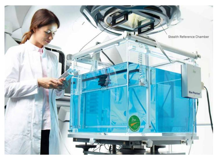
**Blue Phantom**<sup>2</sup> filled with AquaBlue, a special water treatment for protecting mechanical parts and protecting water from decay.
