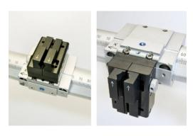
The Universal Detector Holder allows stable and reproducible setup of detectors in the IBA WP-Systems, both horizontally and vertically.
