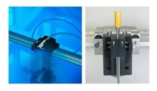
The horizontal orientation is shown with the mounting of the CC13 Ion-Chamber. The vertical orientation is demonstrated with the mounting of the RAZOR™ Diode.
