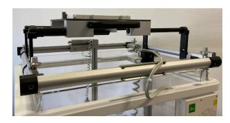
Stealth reference chamber including special holder for Varian® Halcyon<sup>™</sup> / Ethos<sup>™</sup> (\*) – Linac allows field-size measurements up to max. 28x28 cm without excursions into Linac room for reference chamber re-alignment.
