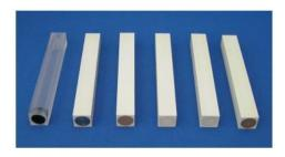
Hollow inserts with 1.7 cm diameter and 16 cm length embedded in 2 cm x 2 cm RW3 block:
