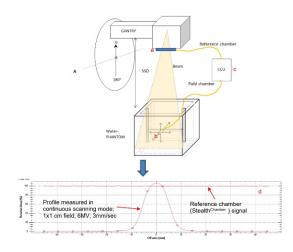
The transmission Stealth™ Chamber (a) mounted with a Stealth holder in the beam, where it does not shadow the field detector for the entire area of programmed positions in order to produce accurate and reproducible scans (d).
