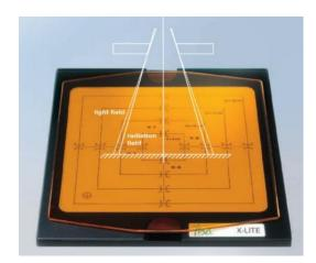
Correct alignment of the light field with the radiation field is essential for reliable treatment set-up. According to national and international recommendations, e.g., NACP (Acta Radiologica Oncology 19 Fasc 1, 1980) and IAEA (Technical Report Series No 277, 1987), this alignment should be checked at least once a week and should correspond to within ± 2 mm at SSD 100 cm.
