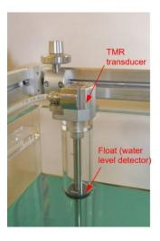
For TPR/TMR measurements, the water reservoir with bidirectional pump must be used. The water pump is controlled automatically by the myQA® Accept software via the CCU.
