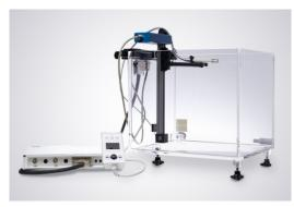
One dimensional, stand-alone motorized water phantom for absolute dose measurements according to AAPM TG-51 (lead filter option needed) and IAEA TRS-398 dosimetry protocols and automated PDDs (myQA Accept 9.0 or higher required).
