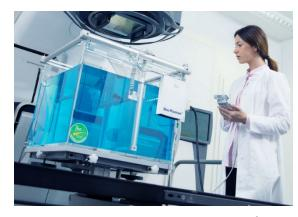
3D Water Phantom System Blue Phantom<sup>2</sup> for complete Linac Commissioning & QA
