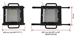
Legs fully retracted and Legs fully extended.
