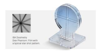
For determination of the isocentric accuracy. The film is held between the two perspex disks and a tool provided defines the center of crosshairs on the film.
