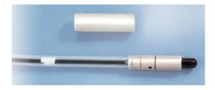
Waterproof, ventilated thimble chamber suitable for electron and photon beam dosimetry. Supplied with a 60Co factory calibration certificate  $(N_{D,W})$  traceable to PTB.
