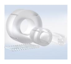
Adult Head & Body / Pediatric Head Body Innovative 3-part nested PMMA phantom CTDI for measurements. Designed to image pediatric and adult head and body in accordance with FDA performance standard for diagnostic X-ray systems (21CFR 1020.33).
