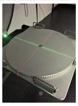
The handles on the turntable enable convenient and safe transport and positioning on the patient table:
