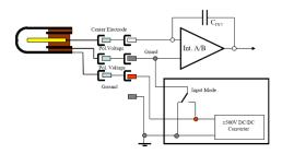
The conventional system, e.g., "grounded input," clamps the electrometer amplifier and center electrode of the chamber on ground potential and provides the polarization voltage to the outer chamber wall.
