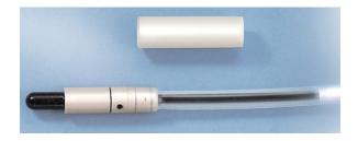
Waterproof, ventilated thimble chamber suitable for quality assurance in air and for low dose measurements in water phantoms. Supplied with a 60Co factory calibration certificate (N<sub>D,W</sub>) traceable to PTB.
