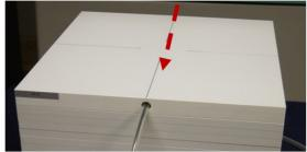
Plan Parallel PPC05 inserted in the adapter plate:
