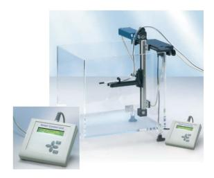
One dimensional, stand-alone motorized water phantom for absolute dose measurements according to AAPM TG-51 (lead filter option needed) and IAEA TRS-398 dosimetry protocols.
