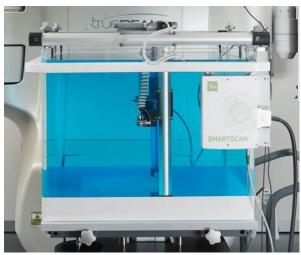
3D Water Phantom System SMARTSCAN for complete Linac Commissioning & QA
