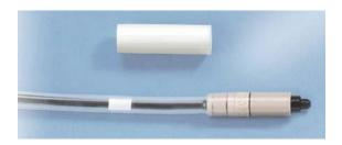
Waterproof, ventilated thimble chamber for relative dosimetry, absolute dosimetry, especially for stereotactic, IMRT or any small field measurements.
